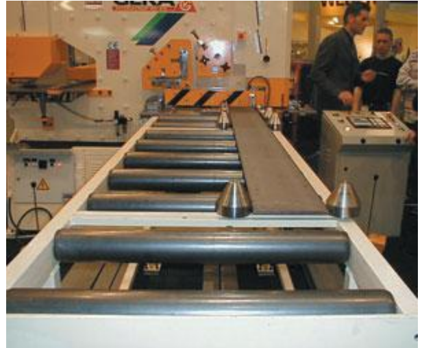
This full ironworker has an X-Y coordinate CNC punch positioning table and a CNC
