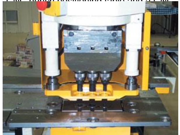
This triple-gag punch has a hydraulic stripper mounted with an X-Y coordinate CNC punch positioning table.
